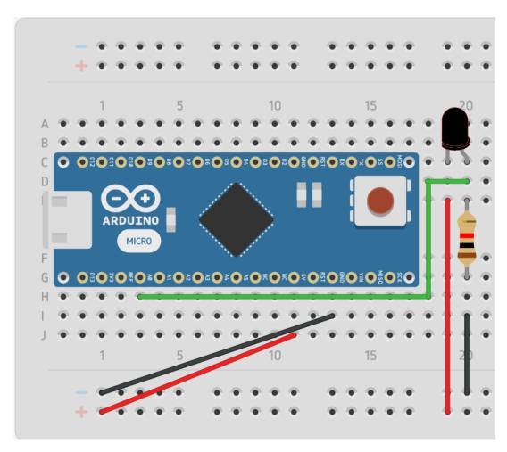
Note: If you get no reading when igniting a flame near the sensor, try reversing it. It is a polar device and needs to be in the correct way. It will not be damaged in this circuit if it is placed backwards.
