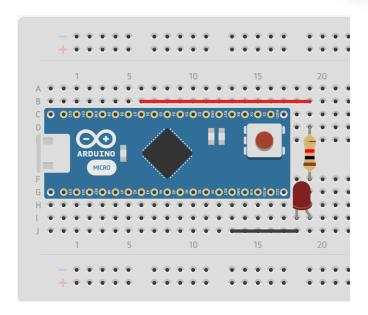
Note: The LED will not be damaged if it is placed in backwards, however it will not light until it is swapped to the correct direction.
